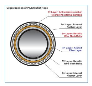
The PILER ECO Hose, which is inserted into the ground with a pile was developed exclusively to be extremely durable with high anti-abrasivity and tensile strength.
